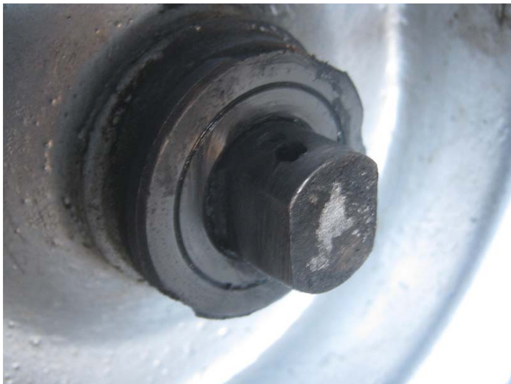
#2 shows cut axle. Axle was cut with super thin cutting disc on angle grinder.
