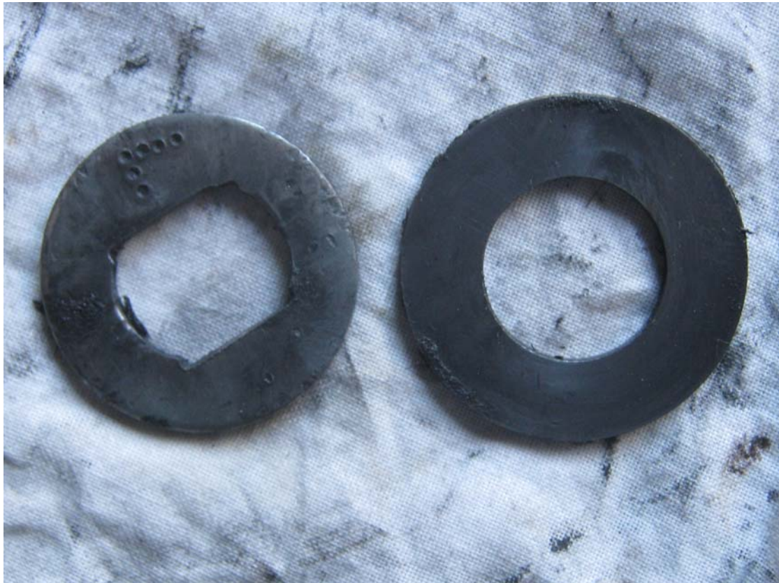
#4 Both washers shown. First is rotating 'rub' washer. 2nd is fixed 'thrust' washer. Second washer MUST be a neat shaped fit to the cut axle. Grease MUST be applied
